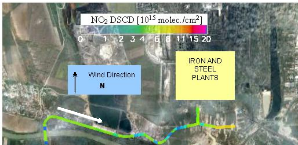
Figure 6. The NO 2 DSCD near the iron and steel plants in Galati city
